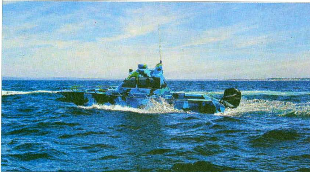
A.F. Theriault and Sons Ltd. in Meteghan River has created a mid-water patrol boat featuring a hull of ceramic-reinforced plastic, which a company official says is 'the result of five years of intense R&D work . . . that emanated from the 9-11 crisis in the States.' (Contributed)
