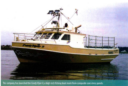
The company has launched the Fundy Viper II , a high-tech fishing boat made from composite core stress panels.
